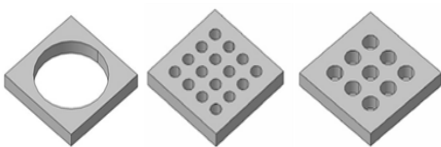
Fig. 4. The orifice models used in the internal passage
