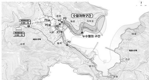
Fig. 5. Leakage candidate pipes in A district
