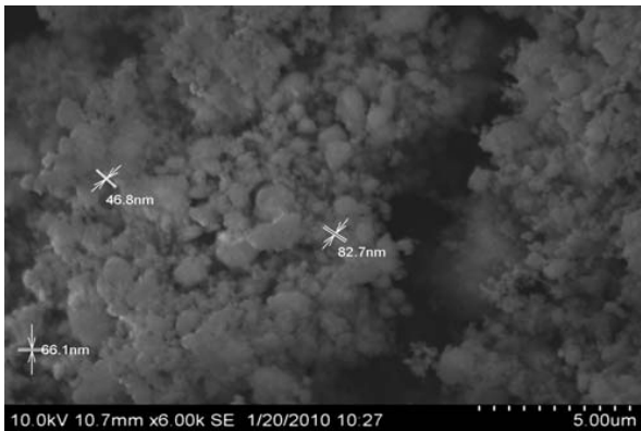
Fig. 2. SEM analysis of nano sized alumina
