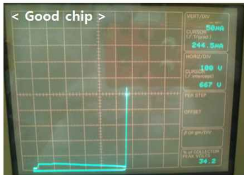
Fig. 14. Breakdown voltage measurement of 600 V/2A trench filling super junction MOSFET.
