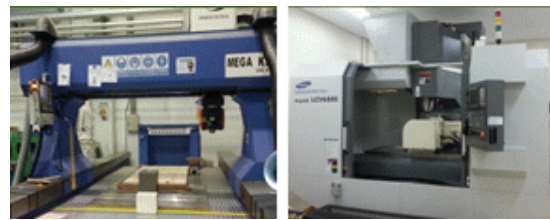
Fig. 2 Two different types of 5-axis machine tool for accuracy evaluation(Head-tilt and Table-tilt type)
