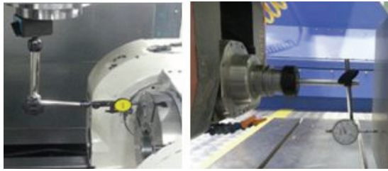
Fig. 3 Accuracy measurement of 5-axis machine tool
