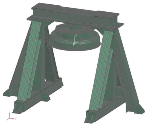
(a) Finite element model for mirror cell assembly
