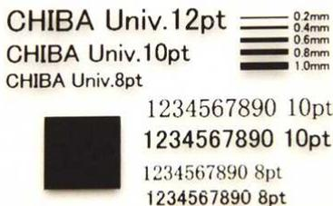
**Fig. 16. Photograph of ink-jet printed image on glass.**
