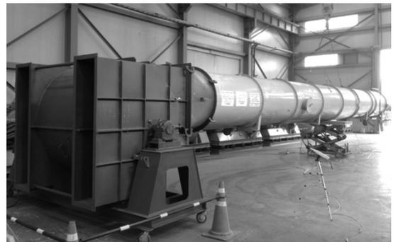
Fig. 2 Reference blower and blower performance tester
