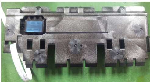
Fig. 5. Semiconductor optical filter module assembly for financial account information recognition.
