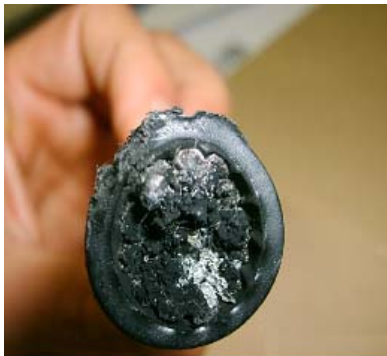
Fig. 2. Photo of depleted cable.
