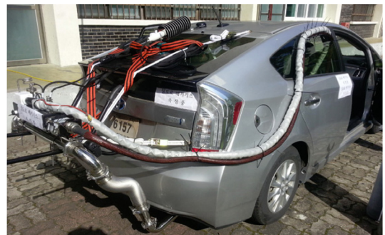
Fig. 3 Photograph of test vehicle equipped with PEMS
