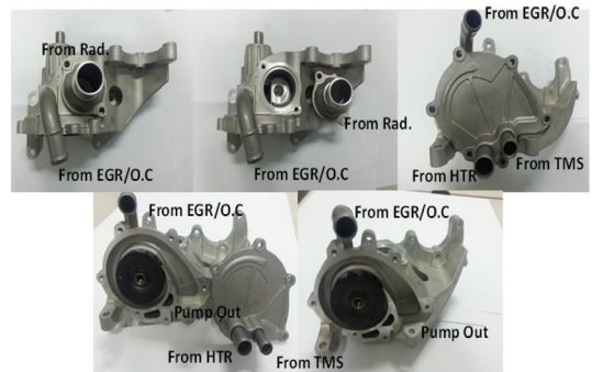
Fig. 2 Photograph of a water pump and inlet pipes
