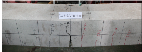
Fig. 5 Crushing failure mode for specimen EN-45-400
