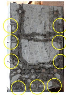
Fig. 10 Beam section by saw-cut
