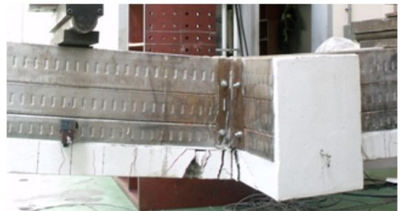
Fig. 9 Concrete cracks of negative moment test
