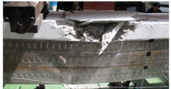
Fig. 8 Concrete crushing of positive moment test
