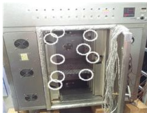
Figure 2. Temperature measuring device for QRD microwaves and positions of QRD microwave magnetrons (Left: 5 kW, Right: 4 kW).
