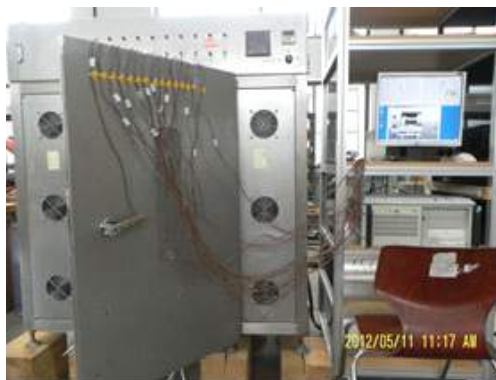
Figure 2. Temperature measuring device for QRD microwaves and positions of QRD microwave magnetrons (Left: 5 kW, Right: 4 kW).
