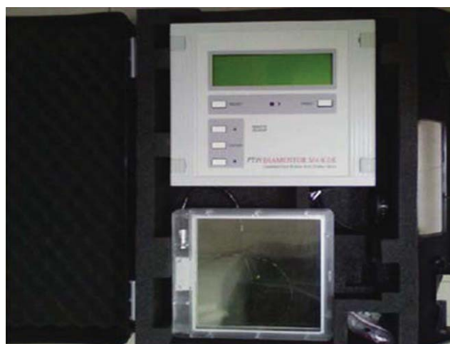
Fig. 1. DIAMENTOR M4-KDK (PTW, Freiburg, Germany) used for the measurement of DAP.
