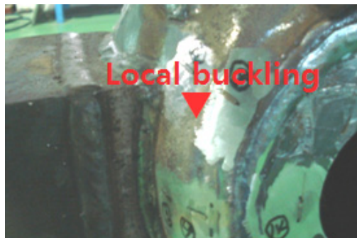
(b) Bottom opening under compressive force
