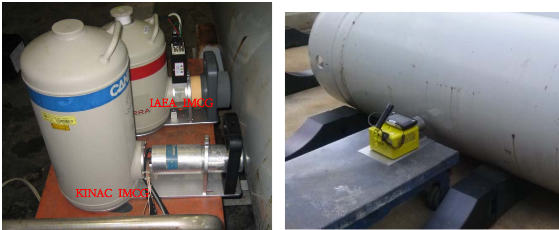
Fig. 4. Measurement of UF_6 cylinder enrichment using IAEA IMCG, KINAC IMCG and portable hand-held HPGe.
