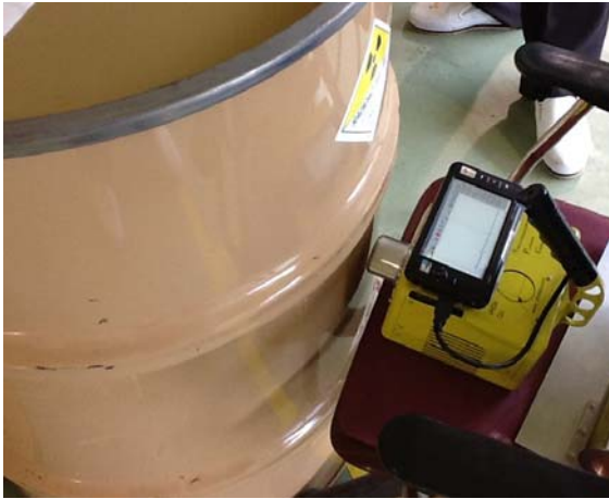
Fig. 5. Measurement of natural UO_2 powder enrichment using portable hand-held HPGe.
