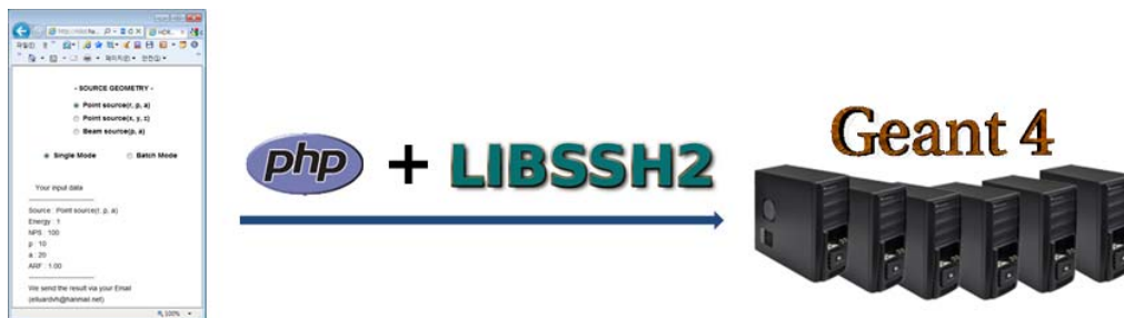
Fig. 4. Scheme for linking web sever to cluster sever by using PHP and LIBSSH2.
