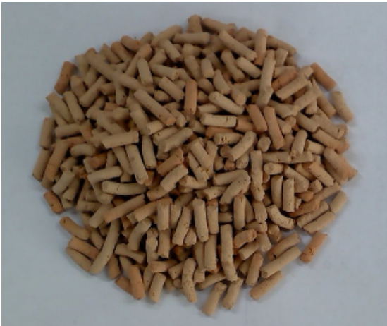
Figure 1. Pellet-type adsorbents prepared from water-treatment sludge.
