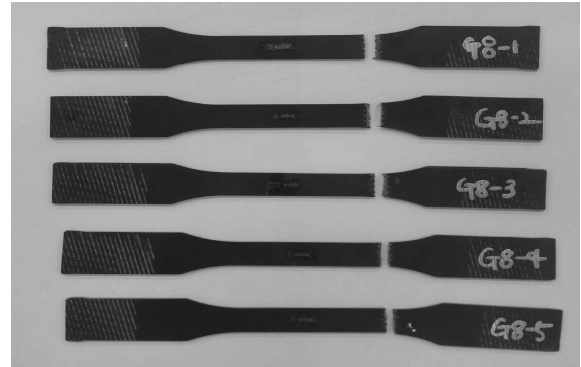
Fig. 9 Failure Patterns of Fabric Tensile Test Specimen
