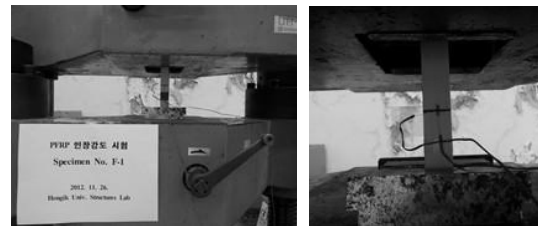
Fig. 3 Tensile Tests of PFRP
