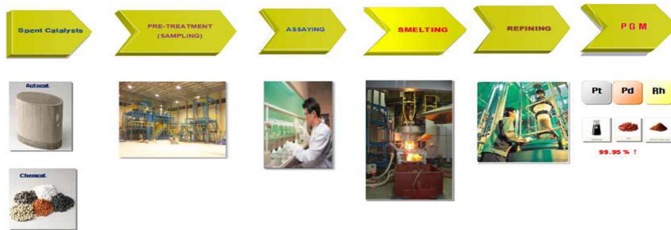
Fig. 2. Recycling processes for spent autocatalyst in 'HeeSung PMTech' in Korea
