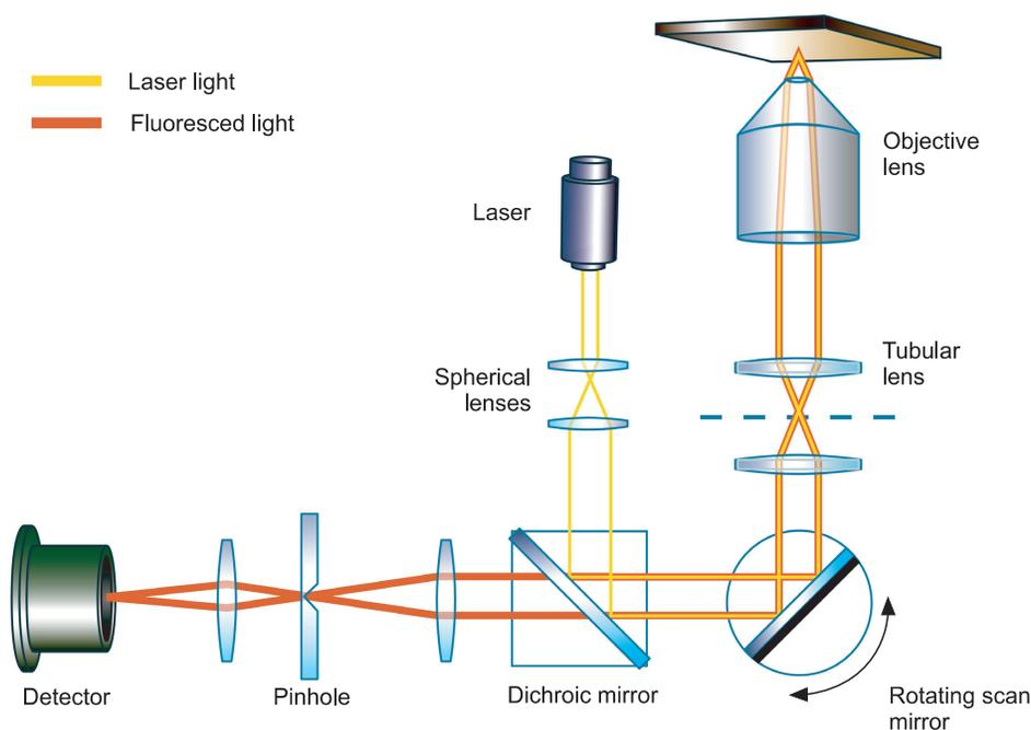
**Fig. 1.** A schematic illustration of confocal microscopy that usually consists of a laser source, microscope (a series of lenses), detector, and pinhole. Fluorescent dyes are used to track individual molecules.
