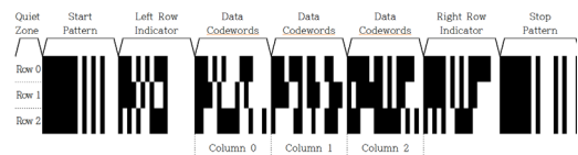
[Fig. 2] Structure of PDF417 barcode
