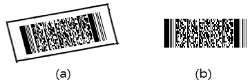
[Fig. 3] Rectification of Distorted Barcode image:
