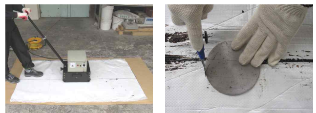
a. Heating the joint part b. Hydrostatic specimen
