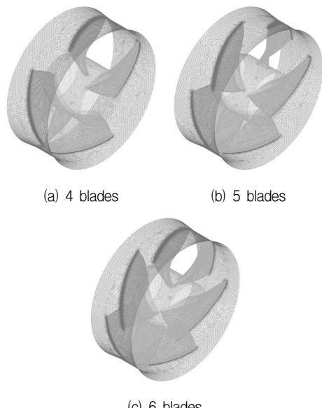
Fig. 2 Numerical grids of three of runner vanes
