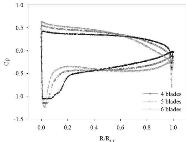
Fig. 14 Pressure coefficient distributions at 50% section of runner vane (120% flow rates)
