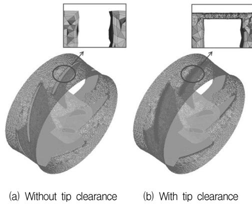
Fig. 3 Numerical grids of runner vane of 10kW class propeller turbine
