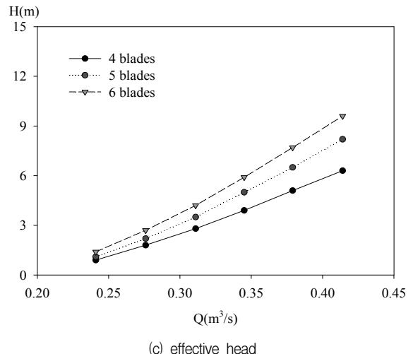
Fig. 8 Performance comparison curves by various the number of runner vane
