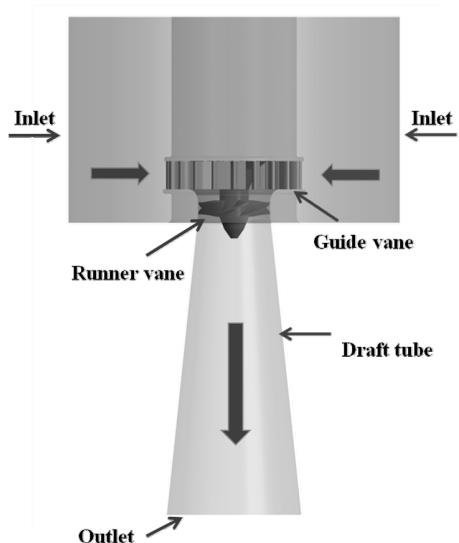
Fig. 1 Schematic view of propeller hydro turbine model
