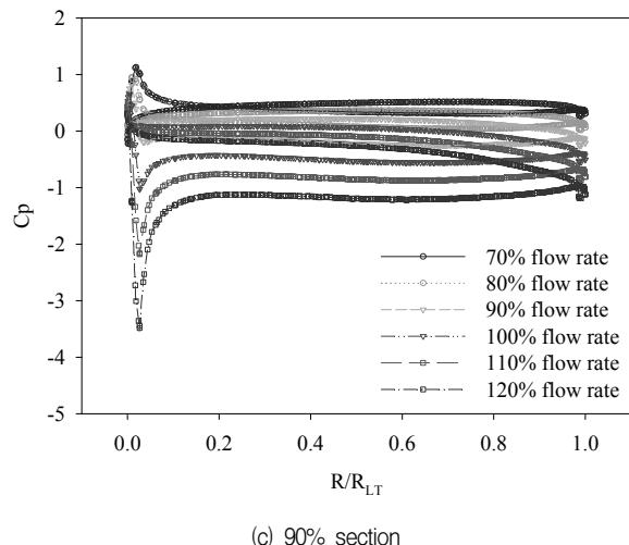
Fig. 7 Pressure coefficient distributions at runner vane sections
