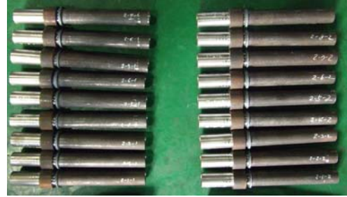
Fig. 2 Friction welded specimen
