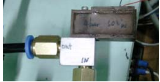
Fig. 7 Fabricated valve for endurance test
