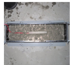
Fig. 5. Dry shrinkage test
