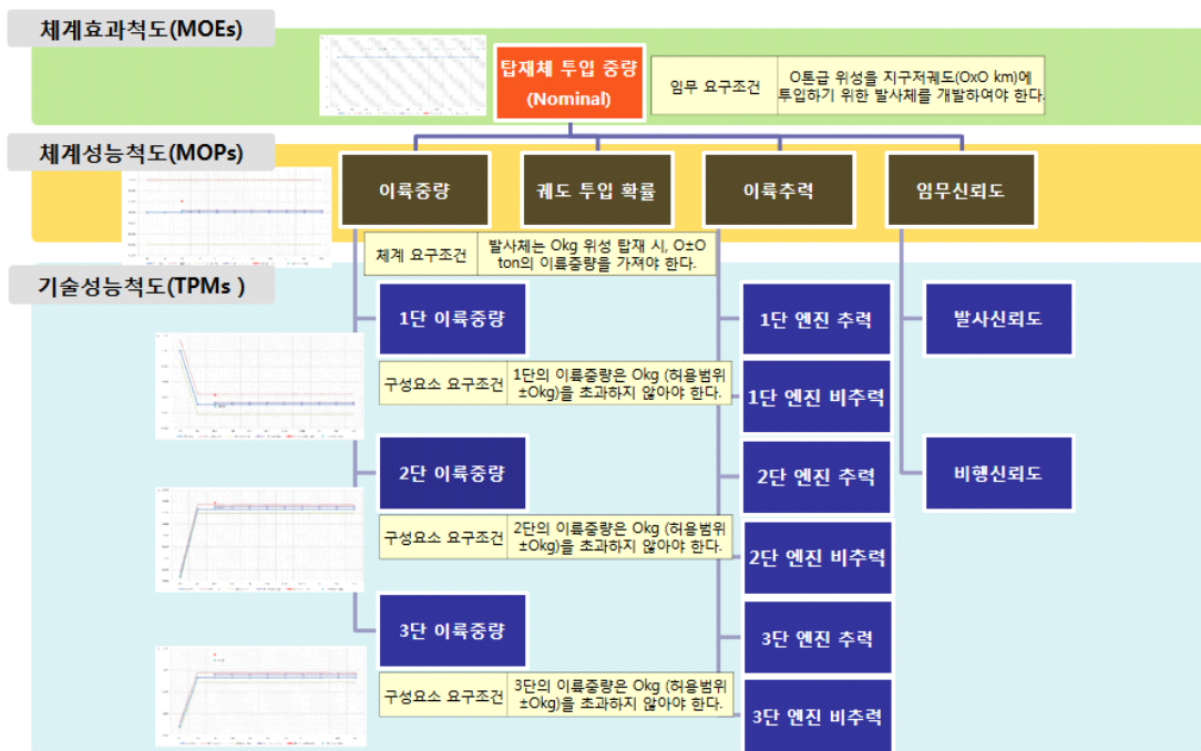
[Figure 7] Hierarchy of technical measures in a virtual space launch vehicle R&D project
