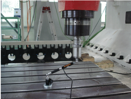
Fig. 6. Calibration experiment using a ball-bar.
