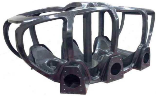
Fig. 4 Manufactured CFRP body frame of CR200
