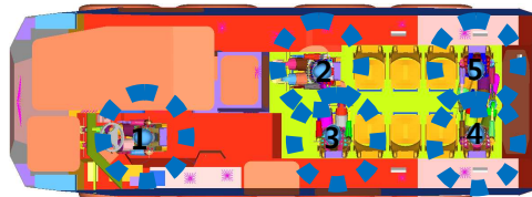
Fig. 5 Location of the dummies for simulations
