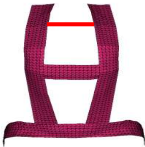
Fig. 8 Addition of an 1D-seatbelt element
