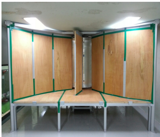
[Fig. 6] The model wind turbine system with the guide vanes and turbine impeller installed at the test section of the subsonic wind tunnel.
