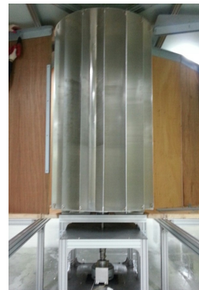
[Fig. 8] The model turbine impeller assembled with 16 blades and mounted on the test
