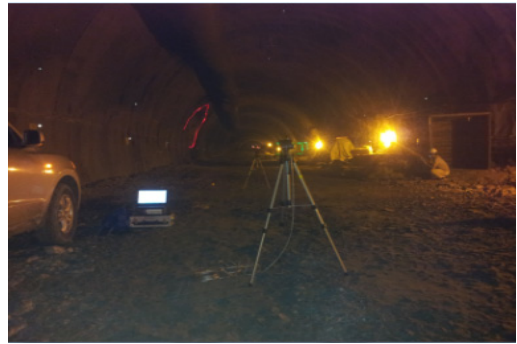
(b) Measurement of sound characteristics using 1/3 Octave Band Analyzer(blasting)
