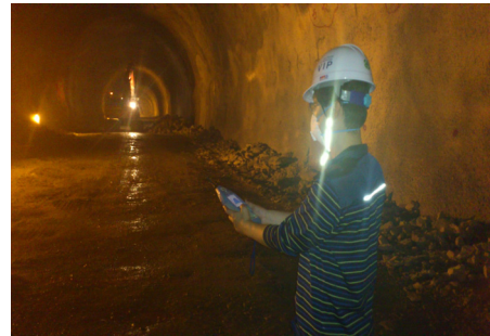
(c) Measurement of sound characteristics using 1/3 Octave Band Analyzer(muck treatment)
