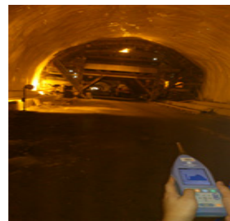
(d) Measurement of sound characteristics using 1/3 Octave Band Analyzer(lining work)
