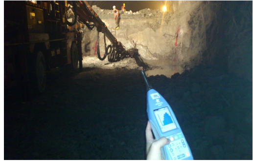
(a) Measurement of sound characteristics using 1/3 Octave Band Analyzer(boring)
