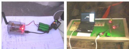
FIGURE 14. USN and mote for data collection
