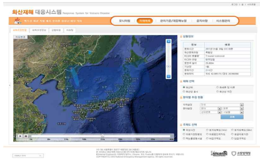
FIGURE 15. Volcanic disaster response pilot system (simulation result of volcanic ash diffusion)
