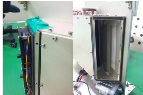
Fig. 6. The isolation of the cooling fan assembly.
