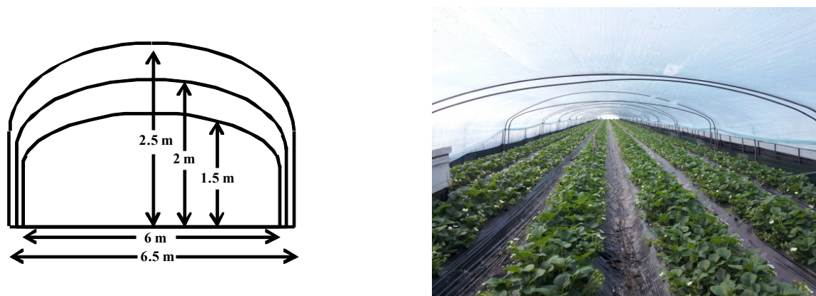
Figure 1. Dimensions (left) and view (right) of greenhouse 1.
