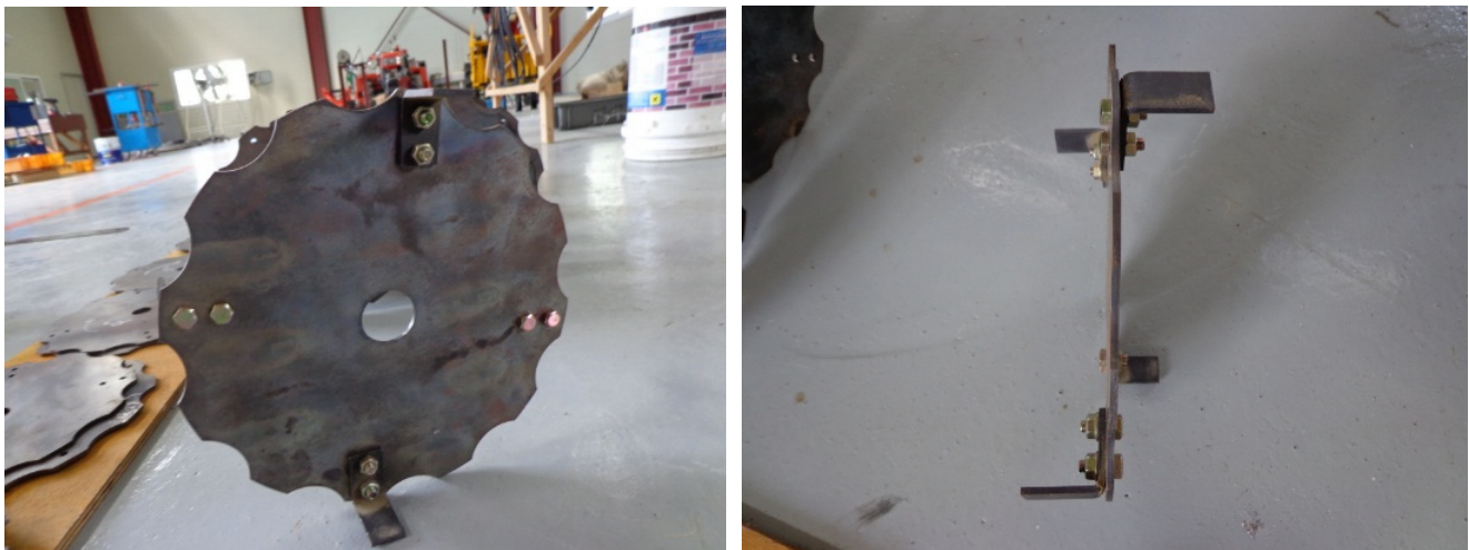
Figure 2. Rotary disk and weeding blade assembly, side view (right) and front view (left).
