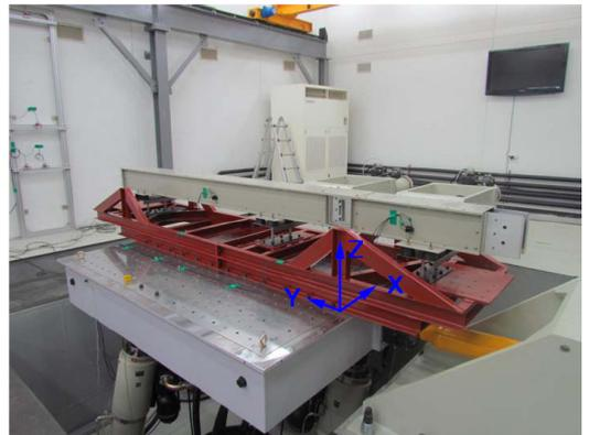
Fig. 13 Seismic & vibration fatigue test set-up
