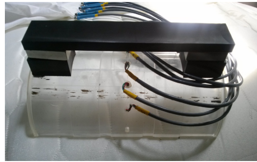
Fig. 5 MFL sensor head for field test
