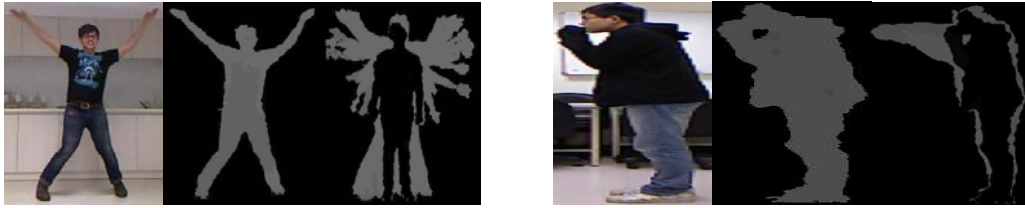
Fig. 4. there are two big columns: left three and right three small columns. From left to right: RGB Image, Depth Map and DMHI of jacking and boxing action respectively
