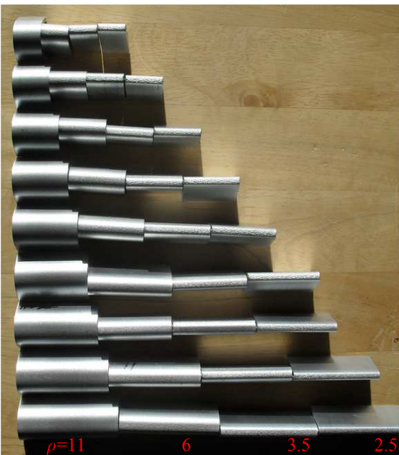
(b) Bending perpendicular to the extrusion direction
