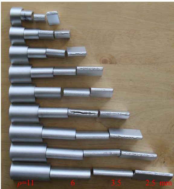
(a) Bending in the extrusion direction
