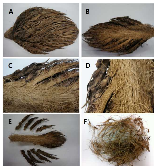
Fig. 2. Morphological Properties of Oil Palm EFB (A: EFB, B: Cross-Section of EFB, C and D: Connected parts of the Core Stem and the branch stems, E: Separated Parts of EFB, F: Shredded EFB).
