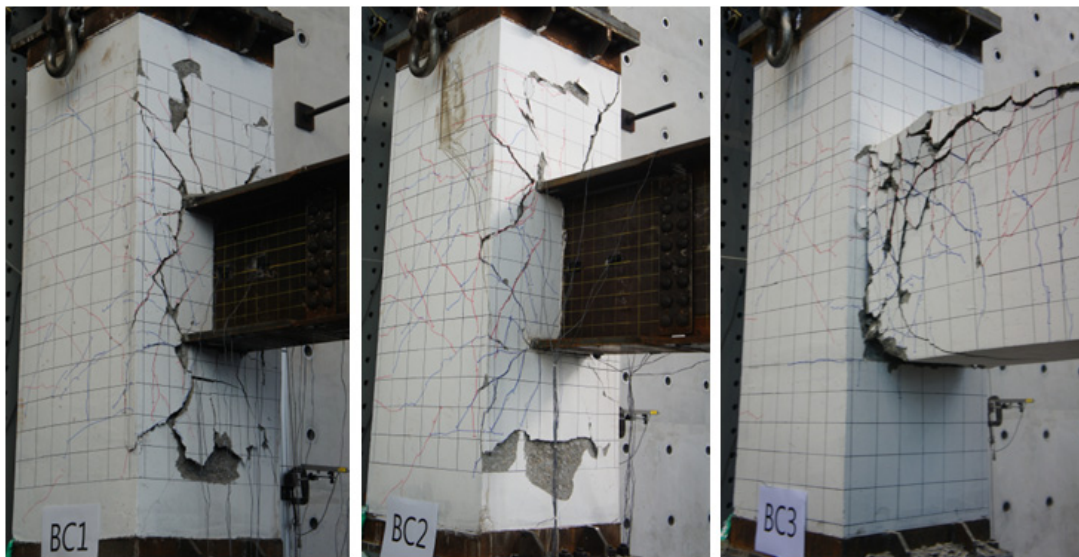
Fig. 9. Damage modes after the end of testing
