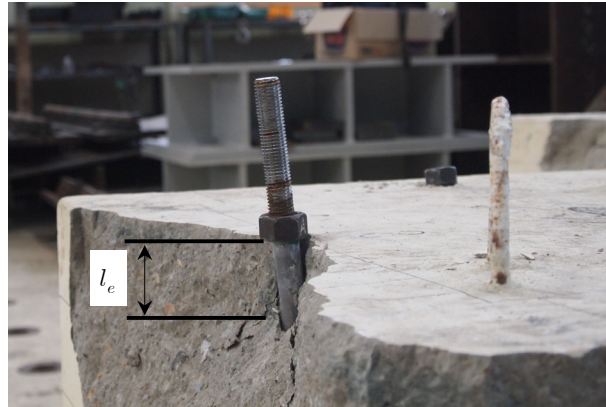
Fig. 14. Definition of bearing depth
