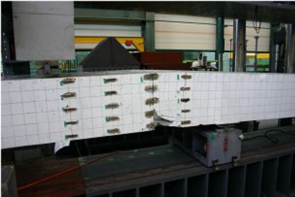
Fig. 6. Failure shape of the beam specimen
