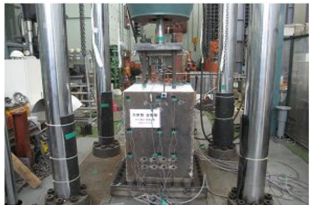
Fig. 5. Test set-up for the tension specimen
