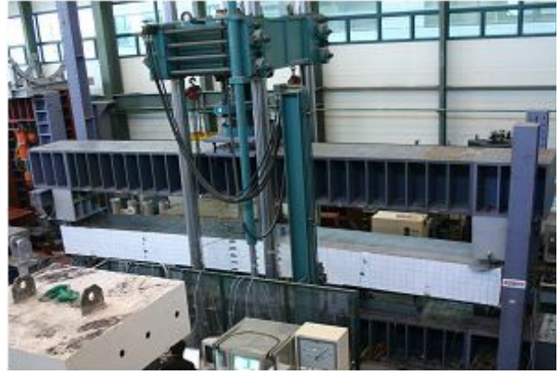
Fig. 4. Test set-up for the beam specimen
