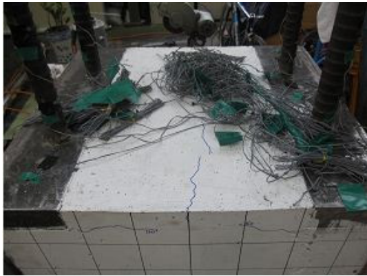
Fig. 15. Concrete crack of the improved form specimen
