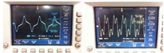
Figure 5: Output waveform by self resonance according to variable frequencies. (Push-Pull topology, turn ratio 2:80, primary inductance(Lm) 3.3uH, Left:300khz/ 2k Vpeak, Right: 265khz/ 2.66kVpeak)
