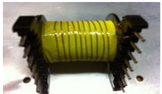
Figure 6: Sparse winding method (1~2mm)
